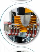
Down-cutting saw blade with Ø 550 mm dia. that rotates between the range of  $45^\circ$  and  $135^\circ$
